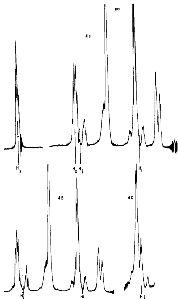
Figure 4.—Nmr spectra of isomer VI: (a) nondecoupled spectra; (b) the H_y proton decoupled from the H_j proton which is now observed as a resolved triplet; 9,10 (c) the H_i proton is decoupled from the H_j proton.
